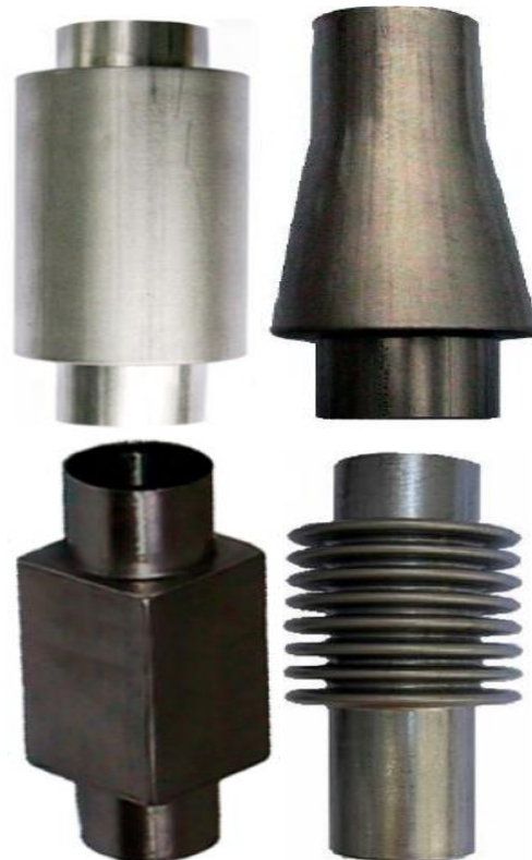
Figure 1. Tube hydroformed parts: (a) cylindrical stepped tube, (b) conical stepped tube, (c) rectangular stepped tube, (d) bellows
